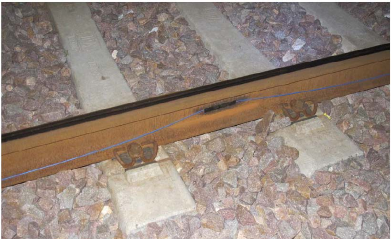
Figure 1: FBG sensor installed on the rail neutral line to detect the temperature change.
