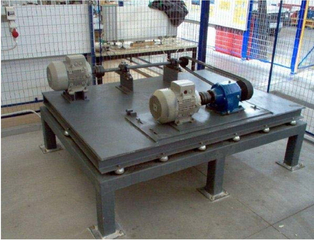
Figure 13. Test rig for the motor startup signal used in section 4.1 (Test case 4).
