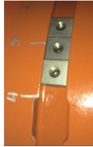
Figure 4: Details of the bearing #8 balance plane and picture of the installed trial weights
