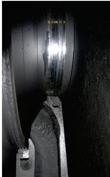
Figure 10: Photos show ferrous sulphide deposits in labyrinth seals.
