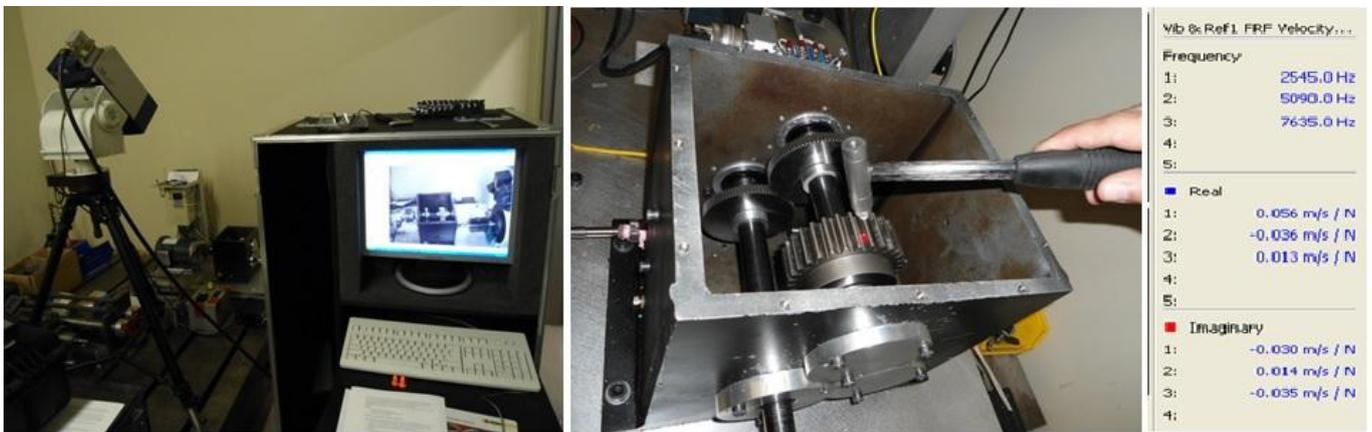
**Figure.3: Modal analysis using vibro-laser and impact hammer.**
