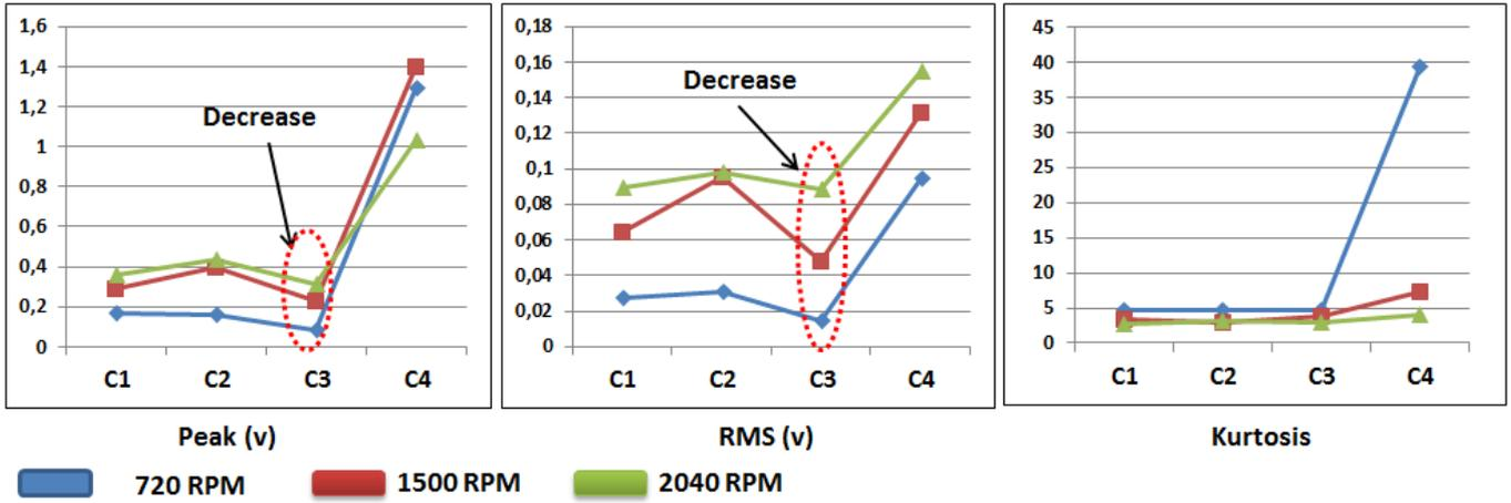
Figure.10: Time indicators: acoustic emission signal.
