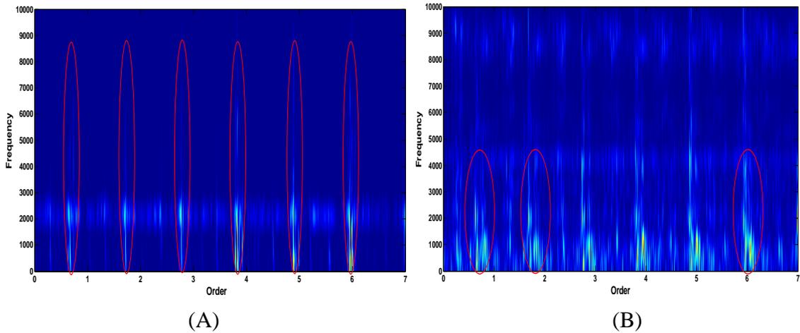
**Figure.9: Spectrogram of defect C4, (A) acoustic emission, (B) Vibration.**
