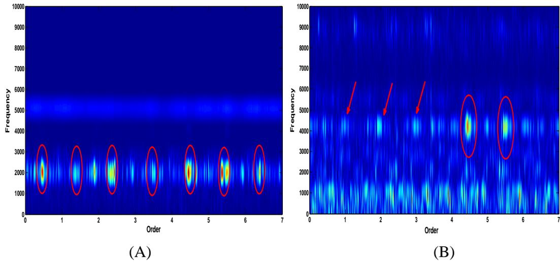
**Figure.8: Spectrogram of defect C3, (A) acoustic emission, (B) Vibration.**
