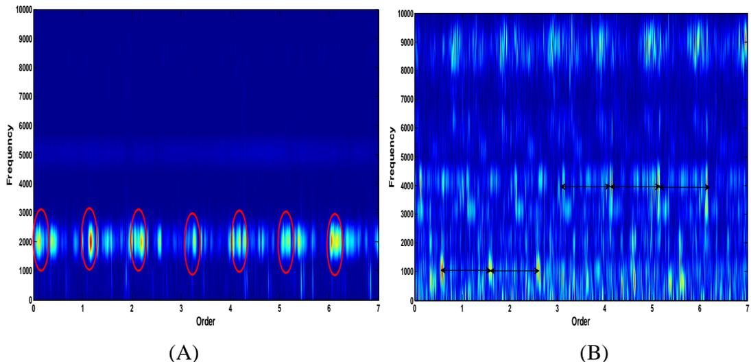
Figure.7: Spectrogram of defect C2, (A) acoustic emission, (B) Vibration.
