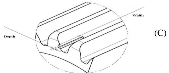
Figure.2 : (A) AE data processing , (B) Heterodyne principle, (C) geometric parameter of the defect.
