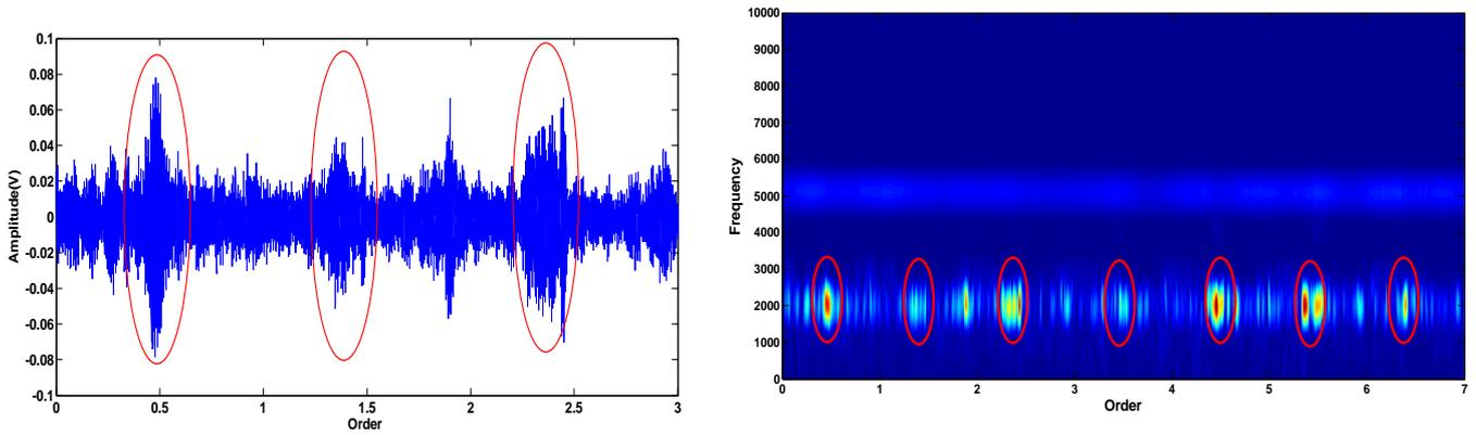
Figure.5: (A) Time signal of defected gear (C3), (B) its spectrogram.
