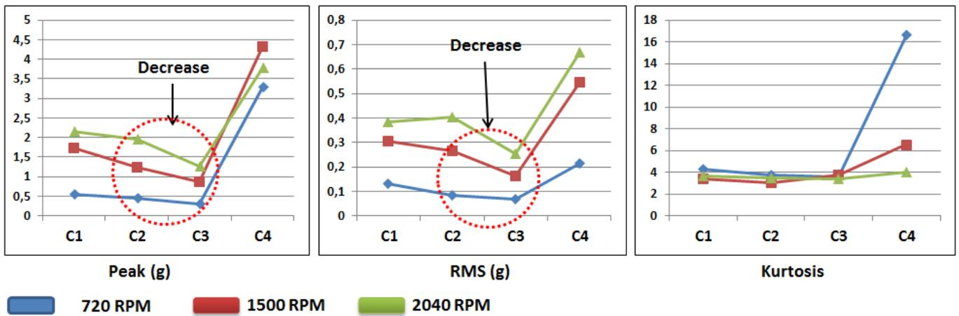
Figure.11: Time indicators: Vibration signal.
