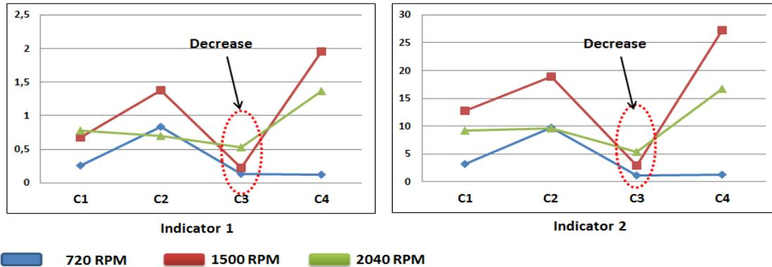
**Figure.15: New indicators applied to vibration data.**
