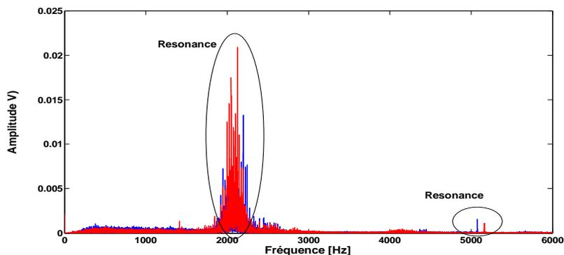
**Figure.4: Spectrum of acoustic emission (recorded at 1500 rpm), blue color for the gear with a light defect (C1), red color for a more advanced defect (C2).**
