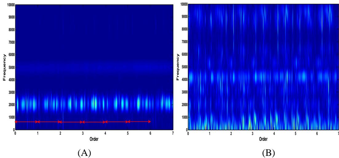
Figure.6: Spectrogram of defect C1, (A) acoustic emission, (B) Vibration.
