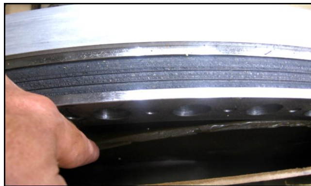
Figure 8: Picture of the wax which was found in the coupling
