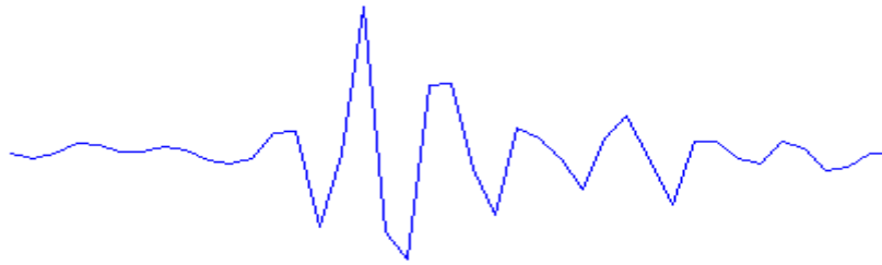
Figure 2: Adaptive wavelet extracted from the signal obtained after UWT and MED filtering
