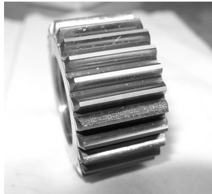
Figure 8: Localized defect in one planet gear wheel.
